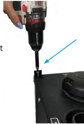
Figure 3b: Anti-tip brackets mounted on top of flow center
