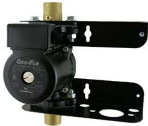
GPM-1 UPS26-99, 230V Grundfos (3-speed), cast iron, iso valves
