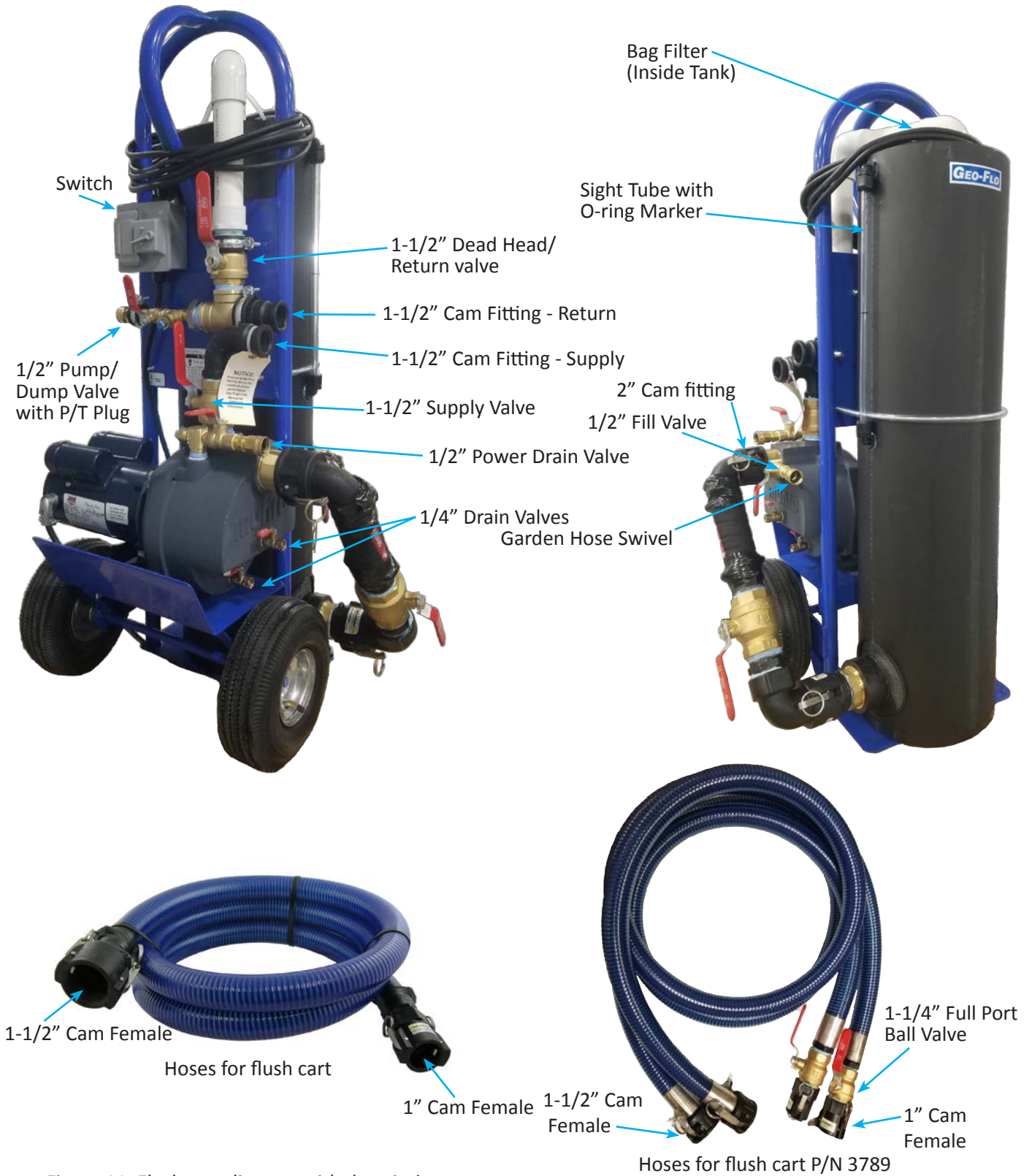
Figure 11: Flush cart diagram with descriptions
